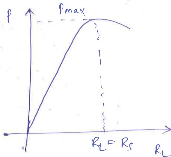
$$\therefore \text{Load power} = I_L^2 R_L$$
