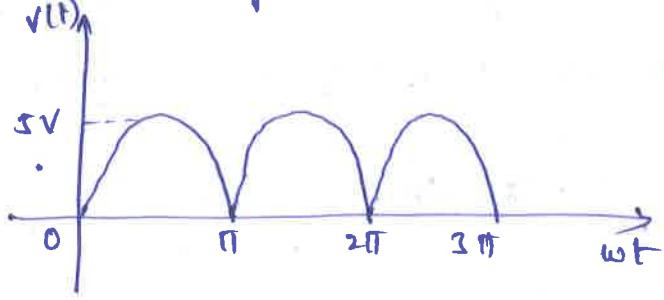
$$V(t) = 5 \sin \omega t \quad 0 < \omega t < \pi$$
