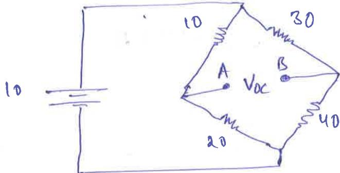
$$\therefore V_{OC} = V_{Th} = V_A - V_B$$
