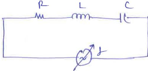
(1) Resonance frequency ( $f_r$ ): The frequency at which the net reactance of the circuit is zero (i.e.) Net reactive power delivered to the circuit is zero
