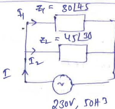
$$(a) I_1 = \frac{V}{Z_1} = \frac{230}{80 \angle 45^\circ} = 7.66 \angle -45^\circ$$
