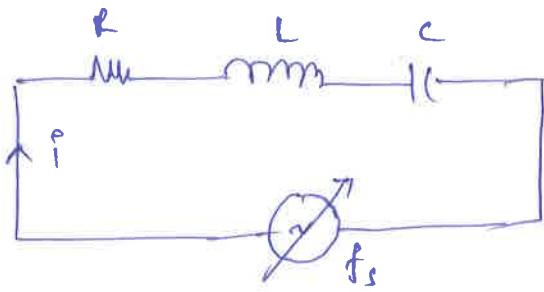
At resonance, Net reactive power delivered by the source / observed by the circuit is zero.
