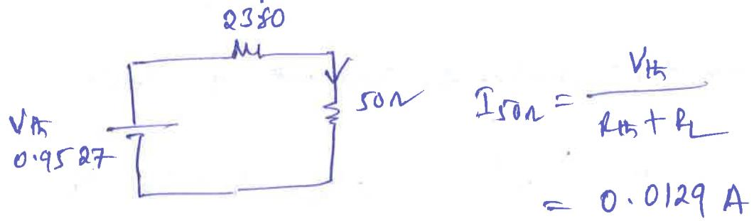
6 (b) Maximum power transfer theorem: In any linear circuit,
